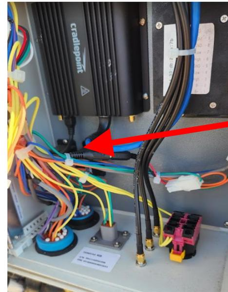
Relays for ECU power and Crank
