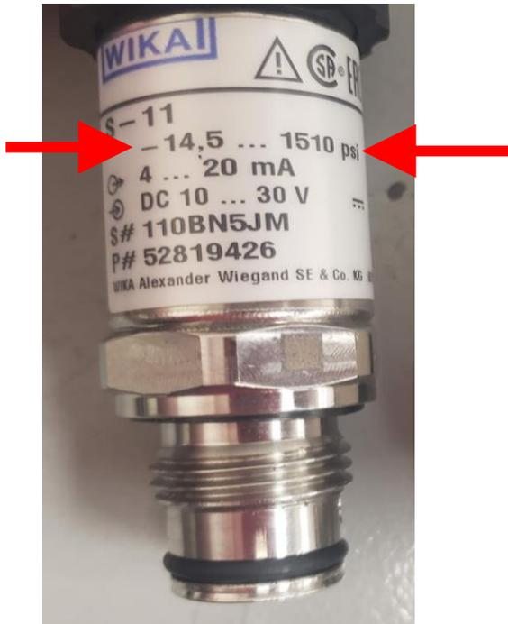
\*Each sensor should have an indicator as to what pressure range it is capable of reading\*
