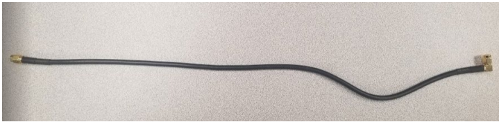
ECS/Nexus internal modem antenna cable 70-1545
