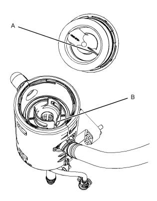
**5.** Install a new filter element into the breather body (3). Ensure the correct position of the element, refer to illustration 90 . Align position (A) on the top cap to position (B) on the filter element.
